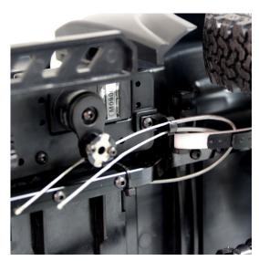
Adjusting the diferential lock controlling wire.
