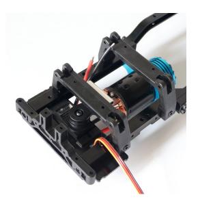
The ESC can be installed beside the steering servo on the front plate.
