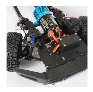
How to install the steering servo.
